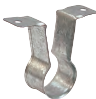
187 (AF 511*) TWO HOLE 90° SIDE MOUNT STRAP SIZE RANGE: ¾" - 2"
