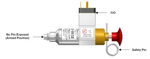
Install the wire lead w/ connector (Item no. 3) to the IVO (Item no. 1) connector and secure with set screw.
