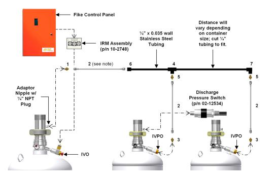
The illustration above shows the items required to make the proper connection between the Container equipped w/ an IVO and the Container(s) equipped w/ an IVPO. The maximum length of pneumatic actuation line (including Hoses) can not exceed 50 ft. (15.2 m) and up to 6 containers equipped w/ an IVPO.
