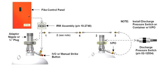
First remove the <sup>%</sup> NPT Plug from Adaptor Nipple, then install Actuation System as shown above. Secure Actuation tubing to a solid surface. Anchoring into plaster, sheetrock wall or any other facing material is NOT acceptable. For additional information regarding the installation and resetting of the IVPO, refer to the IVPO Data Sheet IV.1.10.01
