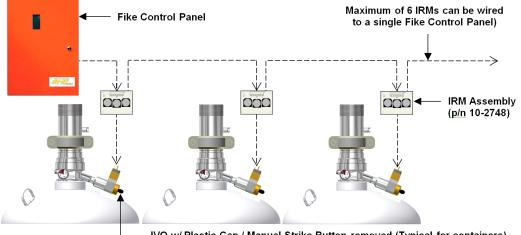
IVO w/ Plastic Cap / Manual Strike Button removed (Typical for containers)
