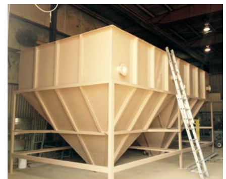
Secondary Clarifier with Chlorination
