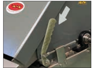
Solids scraper adjustment
